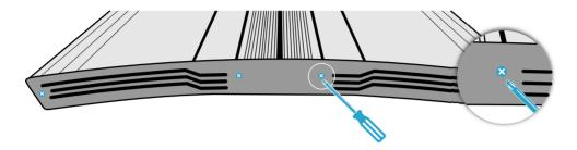
Remove the protective screen by carefully sliding it out.
