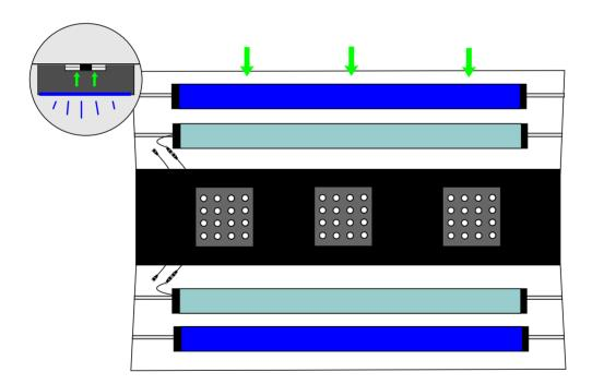
Use the retaining clips provided to clamp them **firmly** between the LED modules in the last third
