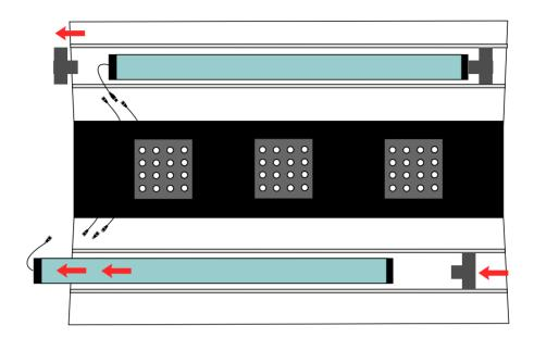
Remove the mounting bracket of the existing LED module by sliding it out, then slide out the LED module and remove the rear mounting bracket.
